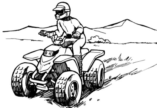
If the rear wheels of your ATV start to slide sideways, control can usually be regained (if there is room to do so) by steering in the direction of the
