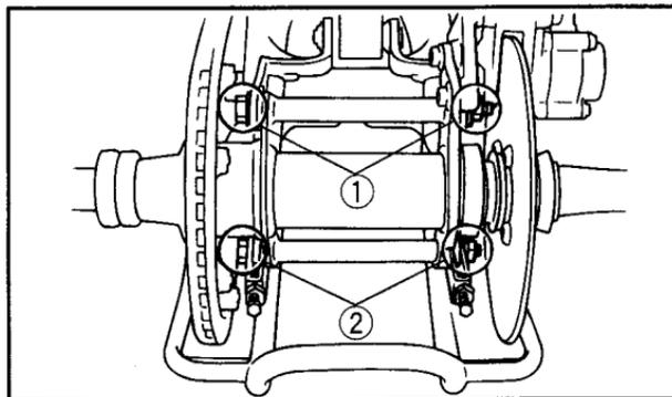
1. Upper wheel hub bolt (x2) 2. Lower wheel hub bolt (x2)
