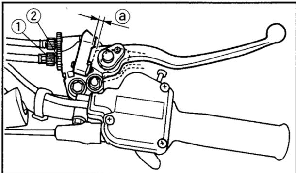
1. Adjusting bolt 2. Locknut a. 3 ~ 5 mm (0.12 ~ 0.20 in)
