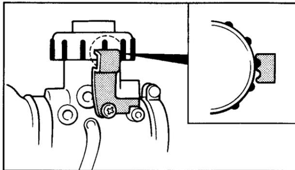
6. Tighten the securing plate screw to the specified torque.
