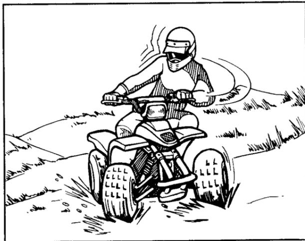
With practice, over a period of time, skill at controlled sliding can be developed. The terrain should be chosen carefully before attempting such maneuvers, since both stability and control are reduced. Bear in mind that sliding maneuvers should always be avoided on extremely slippery surfaces such as ice, since all control may be lost.
