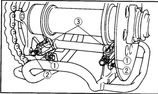
1. Locknut      2. Chain adjuster      3. Alignment marks
