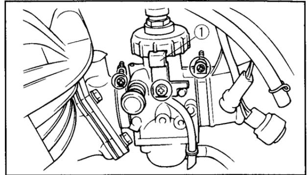
1. Carburetor cap securing plate
