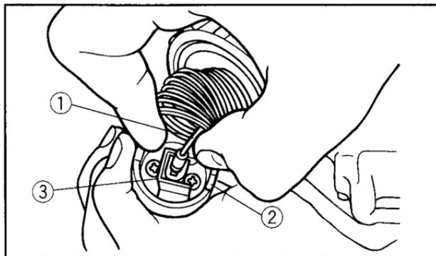
1. Throttle cable 2. Throttle valve 3. Holder
