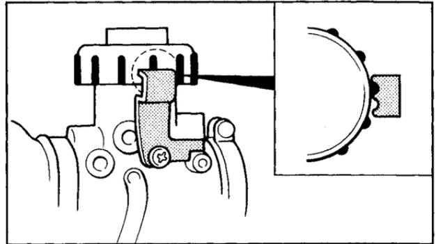
6. Tighten the securing plate screw to the specified torque.
