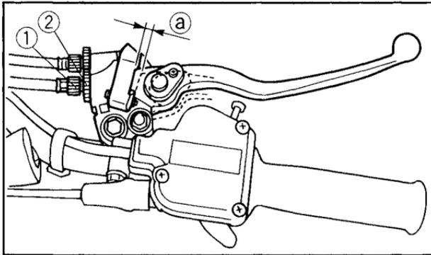
1. Adjusting bolt 2. Locknut a. 3 ~ 5 mm (0.12 ~ 0.20 in)
