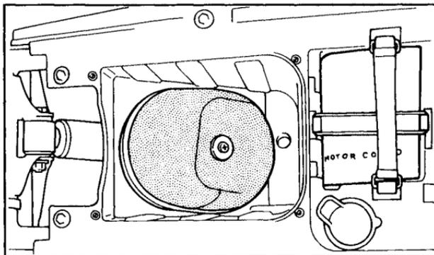
8. Reinstall the element to the element guide.
