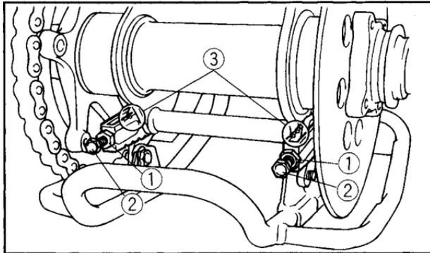
1. Locknut      2. Adjuster      3. Alignment marks
